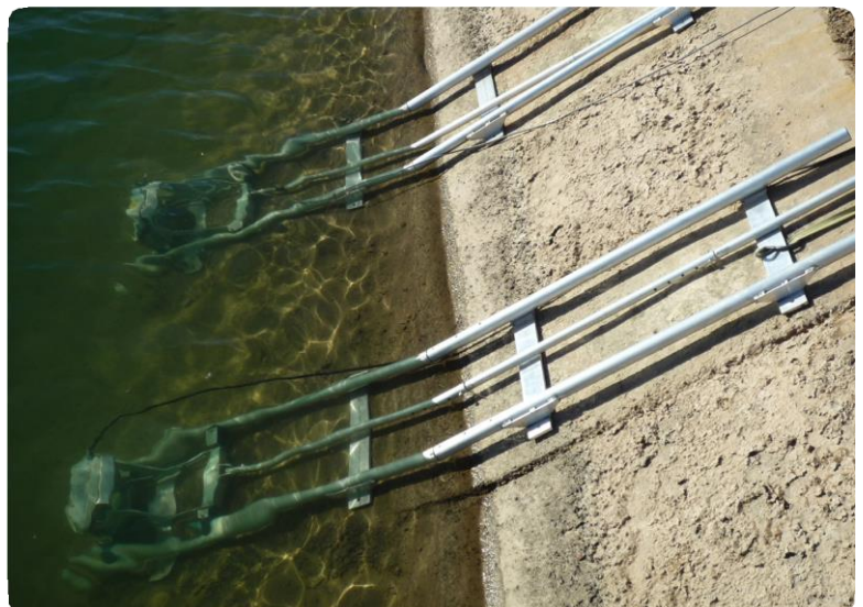
Example of a typical SonTek-SL1500 concrete lined canal installation as part of a HydroMet station.
