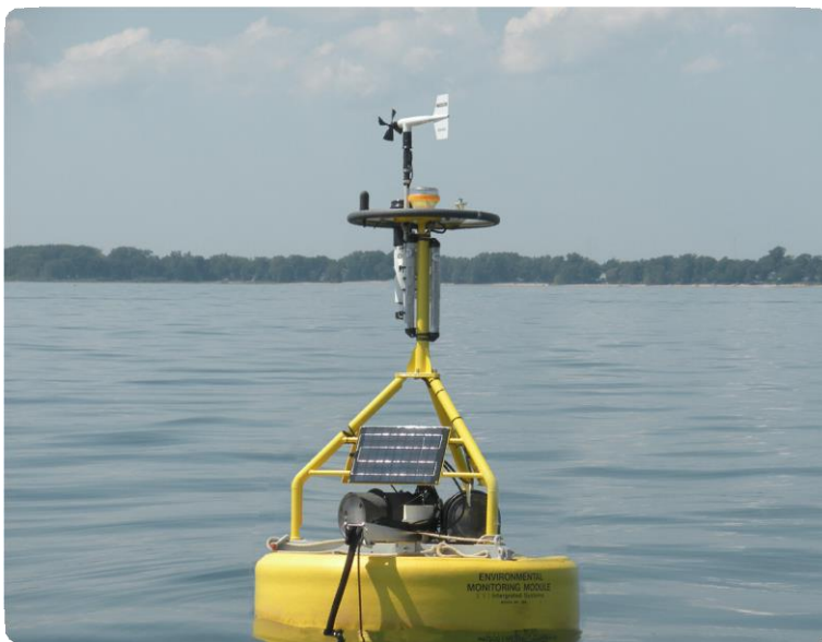
Monitoring Buoy containing meteorological sensors.
