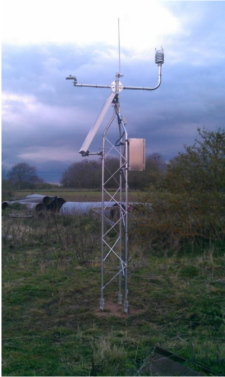
Monitoring tower containing a YSI Data Logger, and meteorological sensors
