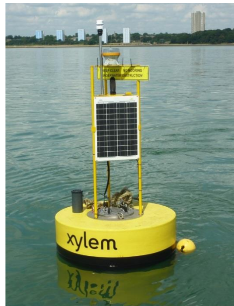
Monitoring Buoy containing meteorological sensors.
