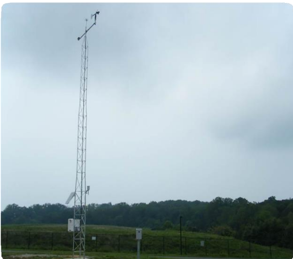
Monitoring tower containing a YSI Data Logger and meteorological sensors
