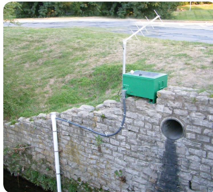
Portable aluminum chest monitoring system containing YSI Sonde and WaterLOG Data Logger. Kansas City, Kansas
