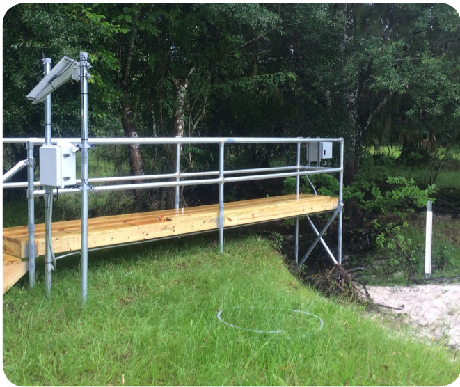
Stormwater monitoring site containing WaterLOG Radar, WaterLOG Data Logger, and Solar Panel. Greenville, South Carolina
