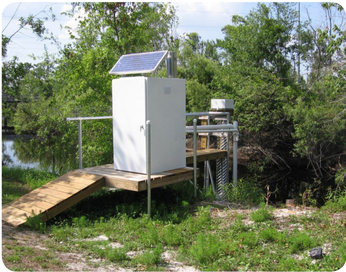
Stormwater monitoring site containing SonTek-SL, WaterLOG Shaft Encoder, YSI level sensor, YSI Sonde, Portable water sampler, WaterLOG Rain Gauge, YSI Data Logger, and Solar Panel. Kissimmee, Florida
