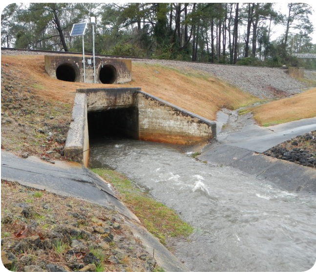
Stormwater monitoring site containing SonTek-IQ®, YSI Sonde, WaterLOG Rain Gauge, Portable water sampler, Customer Data Logger, and Solar Panel. Havelock, North Carolina
