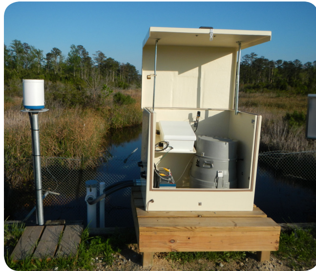
Portable fiberglass clamshell monitoring system containing SonTek-IQ®, YSI Sonde, WaterLOG Rain Gauge, Portable water sampler, Customer Data Logger, and Solar Panel. Havelock, North Carolina
