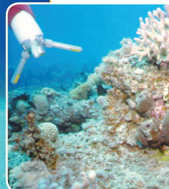
ADV Ocean being used for a near-boundary measurement close to a coral reef.
