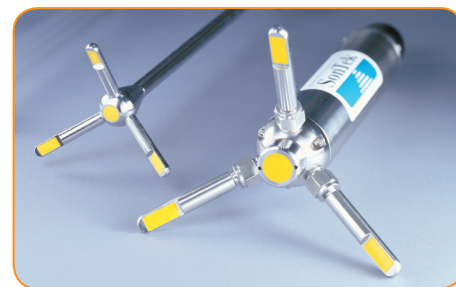
10 MHz ADV on stem with 10 cm distance to sampling volume shown at left. At right is the 5 MHz standard ADVOcean with the stainless steel probe housing.
