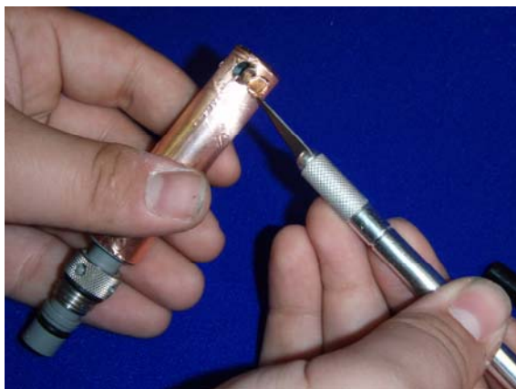
FIGURE 5: Taping pH probe with guard
