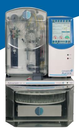
The Aurora 1030W Total Organic Carbon (TOC) Analyzer uses the proven heated persulfate wet oxidation technique to analyze organic contamination levels in aqueous samples. Virtually all organic compounds dissolved in water can be oxidized by heated sodium persulfate (Na $_2$ S $_2$ 0 $_8$ ). Concentrated solutions (1 or 1.5 M) can effectively oxidize organic matter present in the form of colloids, macromolecules, and suspended solids.
