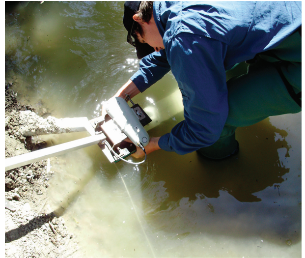
Right out of the box, with just a quick survey of the riverbed and banks input into its onboard software, this SonTek-IQ shallow water flow meter delivered extremely accurate level and flow data.
