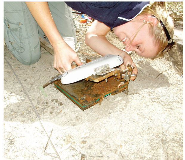
Hydrographer Sophie Gatacre of the NSW Office of Water readies a SonTek-IQ shallow water flow meter for long-term deployment in Colombo Creek. Readings are relayed hourly via modem to her office.
