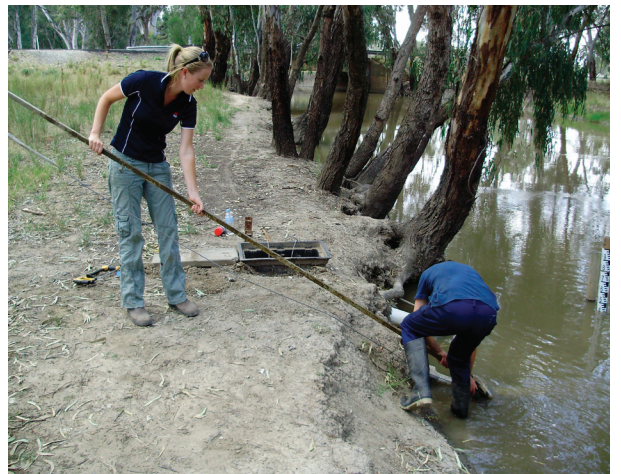
Hydrographers Sophie Gatacre and Simon Turner of the NSW Office of Water adjust the platform under a SonTek-IQ shallow water flow meter, preparing for accurate flow and level measurements in slow-flowing Colombo Creek.
