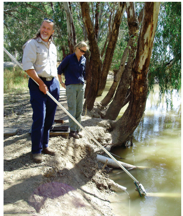
Danny Hannon and Sophie Gatacre of the New South Wales Office of Water deploy a SonTek-IQ shallow water flow meter in Colombo Creek, part of the Murray-Darling river system.
