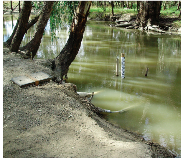
Like the vast network of braided creeks winding through the nearly flat Murray Darling Basin, Colombo Creek in rural New South Wales is highly subject to backwater effects from confluences, trees and other debris, and algal blooms. As a result, gaugings are typically scattered around the rating curve.
