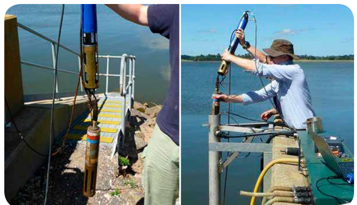
A YSI 6820 suspended beneath an EXO2. Both feed into a CR1000 datalogger which transmits data to an online SCA database.
