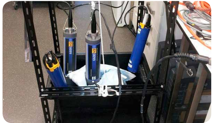
EXO2 Sondes and Legacy 6600-V2 Sondes in pre-deployment quality testing.
