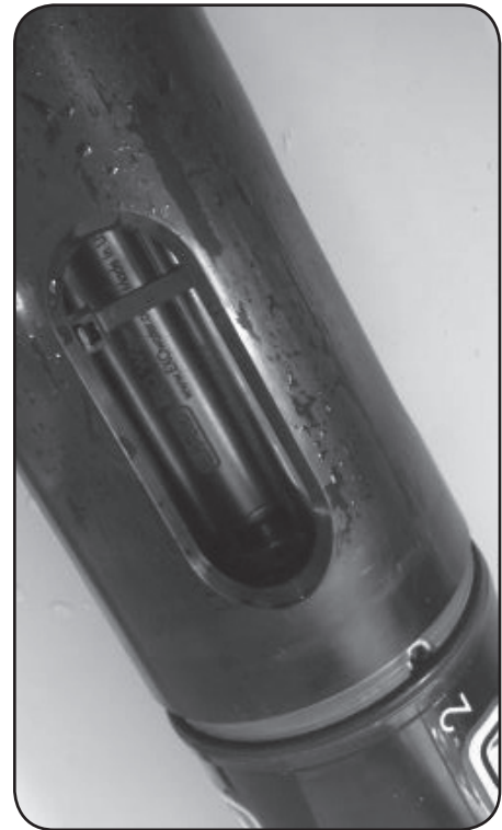
Figure 10 - Place the sensor guard back on to ensure a good fit
