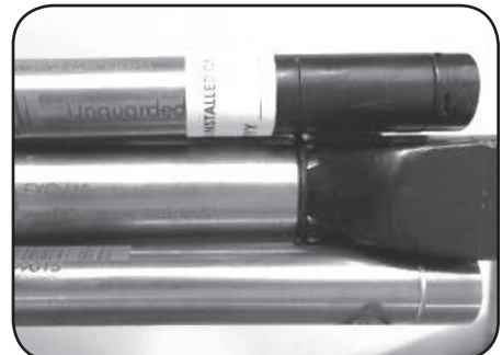
Figure 4 - Sensors installed around the Central Wiper with o-ring in place
