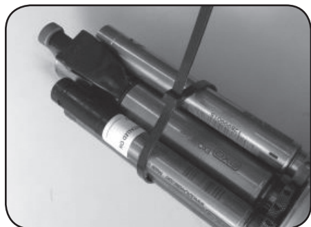
Figure 7 - Securing the sensors with the zip-tie with adequate clearance
