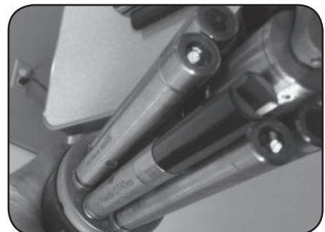
Figure 5 - Wiped C/T sensor in optimal position ready to be secured
