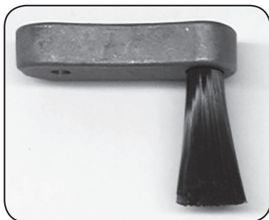
Level 1- New brush, minimal "splay"
