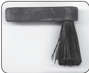
Level 2- Moderate splaying, have spare ready
